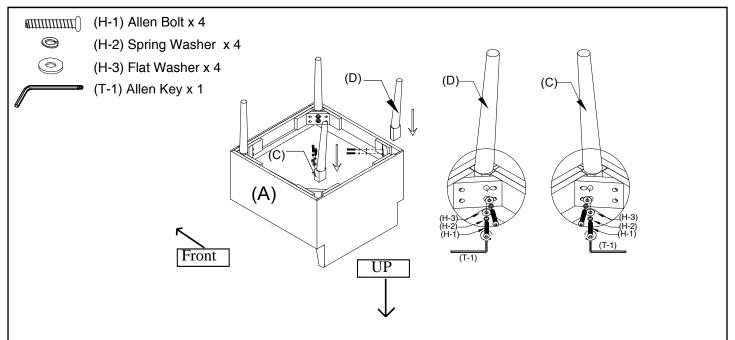
Insert the Right and Left Rear Legs (C and D) into position as shown. The Legs (C and D) are labeled for your convienience. Secure by first engaging Allen Bolts (H-1), Spring Washers (H-2) and Flat Washers (H-3), stacking the hardware in the order shown. Once engaged, fully tighten using the provided Allen Wrench (T-1). DO NOT OVER TIGHTEN.
