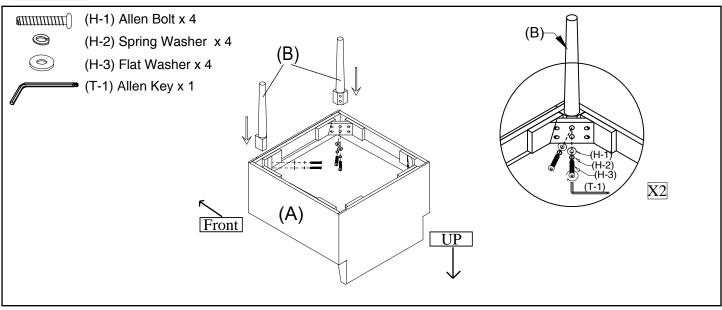
Carefully place Seat (A) upside down on a padded, non-marring surface. Insert the Front Legs (B) into position as shown. Secure by first engaging Allen Bolts (H-1), Spring Washers (H-2) and Flat Washers (H-3), stacking the hardware in the order shown. Once engaged, fully tighten using the provided Allen Wrench (T-1). DO NOT OVER TIGHTEN.
